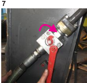
7 B-Quick closing Turn the B-Quick valve clockwise to close it.
