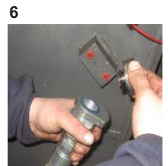
6 Plug the hose with the protection plug
