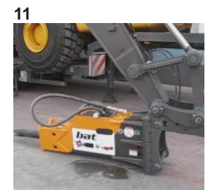
11 Hydraulic Hammer - disconnected from the Excavator
