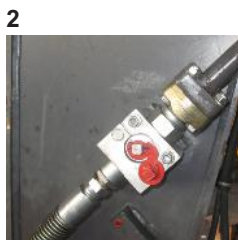
2 Hydraulic hose connected to B-Quick Coupler
