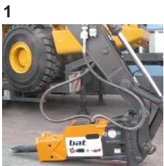
1 Hydraulic Hammer - connected to the Excavator
