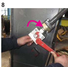
8 B-Quick closing After you insert the plug, turn the B-Quick valve clockwise to close it.
