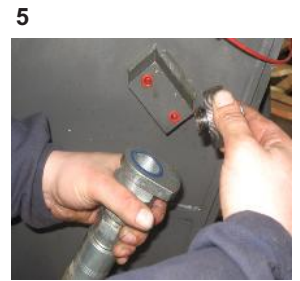
5 Remove protection plug from the Hammer's hydraulic hose
