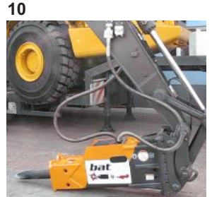
10 Hydraulic Hammer - connected to the Excavator
