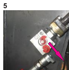
5 Disconnect hydraulic hose from B-Quick
