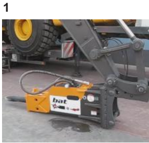
1 Hydraulic Hammer - not connected to the Excavator
