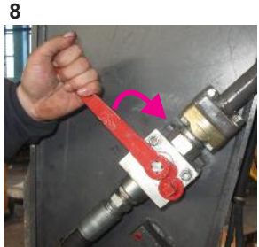
8 Ball valve opening Turn the ball valve clockwise (at the same time, B-Quick is locked)
