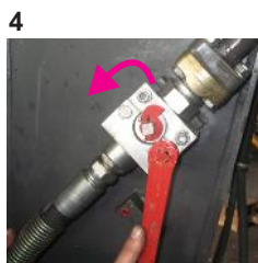
4 B-Quick opening Turn the B-Quick valve anticlockwise to open it.
